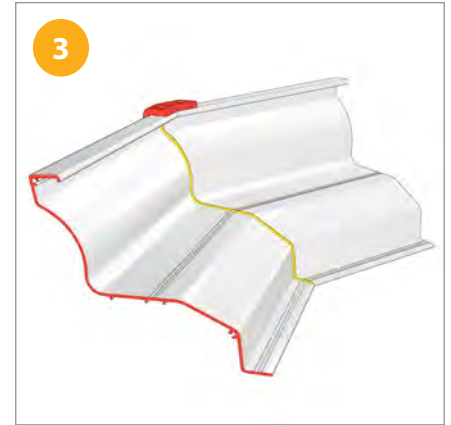
Seal XGUTF-AL1 at mitred joints using low modulus silicone sealant.
