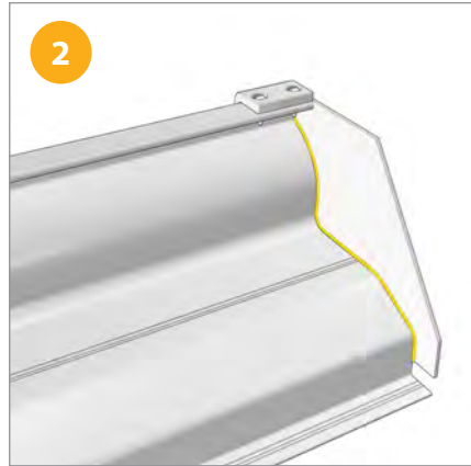
Seal with low modulus silicone sealant in areas shown.
