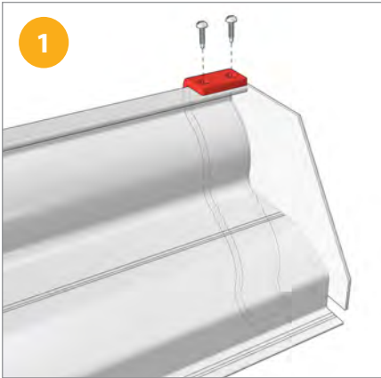
Fix X180E to end of fascia using 2x XM48195SP screws.
